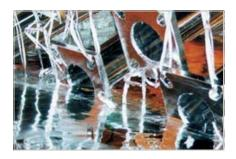
The article is immersed in a bath of molten zinc between 815-850 F (435-455 C). During galvanizing, the zinc metallurgically bonds to the steel, creating a series of highly abrasion-resistant zinc-iron alloy layers, commonly topped by a layer of impact-resistant pure zinc.
